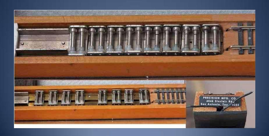
If the model lopes at very low speeds but then runs smoothly with more power, the flexible tubing needs replacement and alignment
