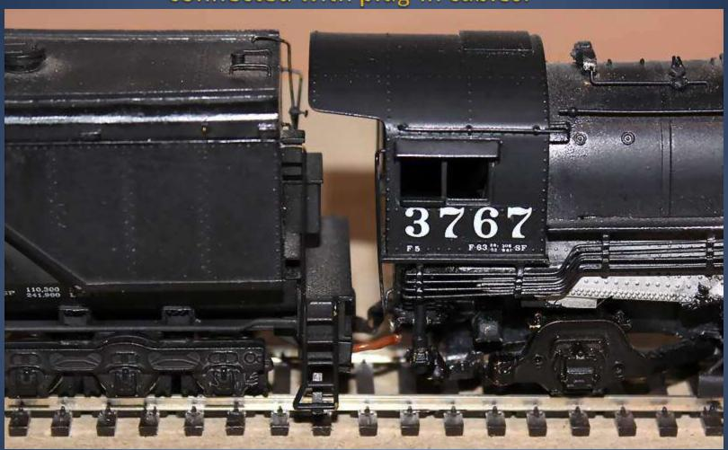
Press on the drivers to see if they are sprung, if one set of drivers does not move, there may be a severe mechanical problem, investigate before testing.
