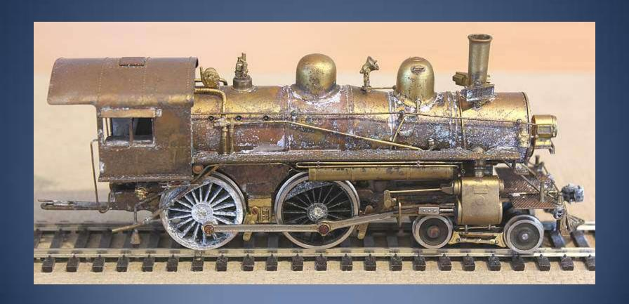
Look for screws that when tightened may rest on a driving axle. Pilot & trailing truck screws are frequent offenders
