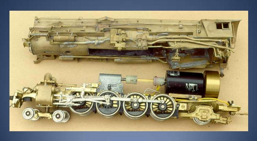
If the model is excessively noisy, it is most likely due to an older, possibly worn out open frame motor or poor gear mesh
