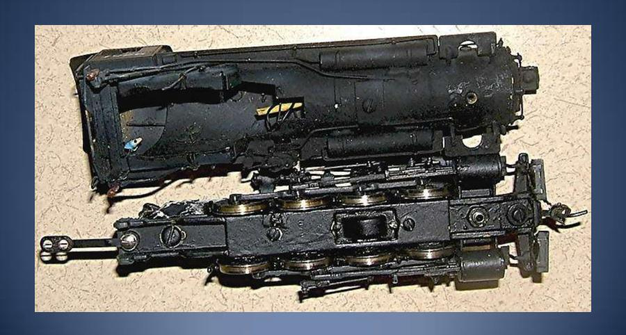
Test just the mechanism with the power supply. If current draw is normal, you missed a problem during the visual inspection
